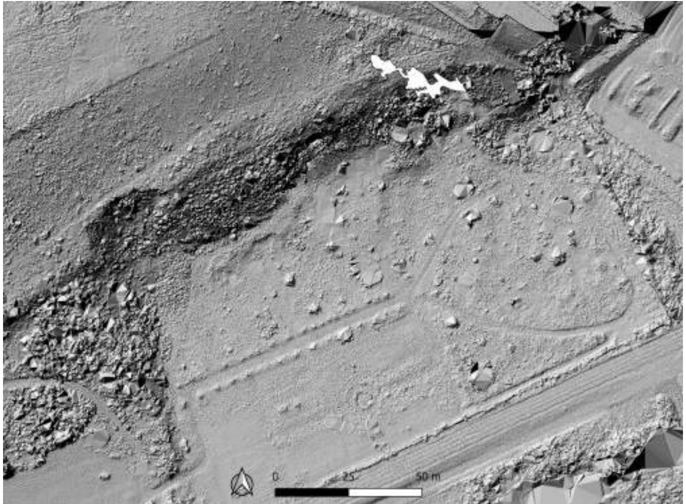
Fig 3. Lidar survey of the site of La Roche-Cotard. Orthophoto. The Lidar image shows the 1846 exploited zone and the cave (LRC I) in white. The cave entrance is in the abrupt northern slope left by workers in 1846. A Lidar drone survey was carried out on the area surrounding the cave using a Yellowscan Mapper, mounted on a Matrice 300 with three passes at a height of 35 m. These scans were then assembled using Yellowscan software. A Digital Terrain Model was generated at 10 cm resolution from these data, along with a hillshade version and contour lines. (Lidar ICONEM).
